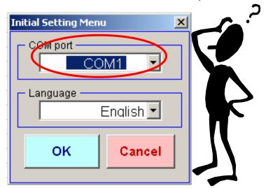
If known select the COM Port for communication. The initial screen provides a drop down selection up to COM 15.
