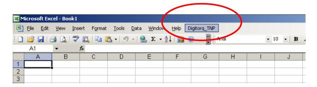
The Digitorq\_TNP menu provides the access for the software. The host PC is now ready to communicate with the TNP Torque Meter.
